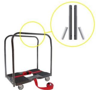
4. Assemble curved bars over Connector Pins in the Hitch. Both sides of bars need to be installed evenly. Bars will be a tight fit so a twisting or shaking motion will assist assembly until Spring Buttons are clicked in place.
